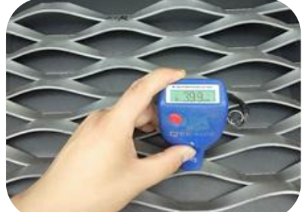
12. Coating thickness testing
